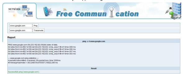
Figure 6-3-1 Network Connectivity Checking
