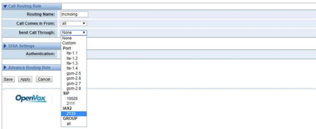
The figure above shows that all the phones in the group ALL are transferred to the IAX2-2133. When the "incoming source" is GSM/LTE port, "prepend", "prefix" and "match pattern" in the "Advanced Routing Rules" are invalid, and only the "CallerID" option is available.
