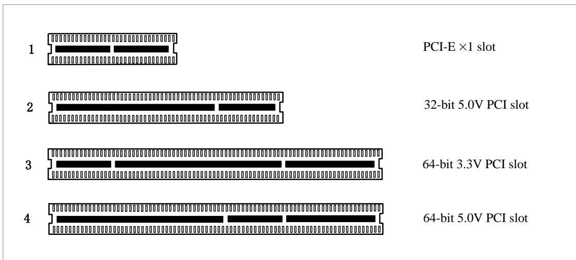
Figure 3 PCI-E and PCI slots
