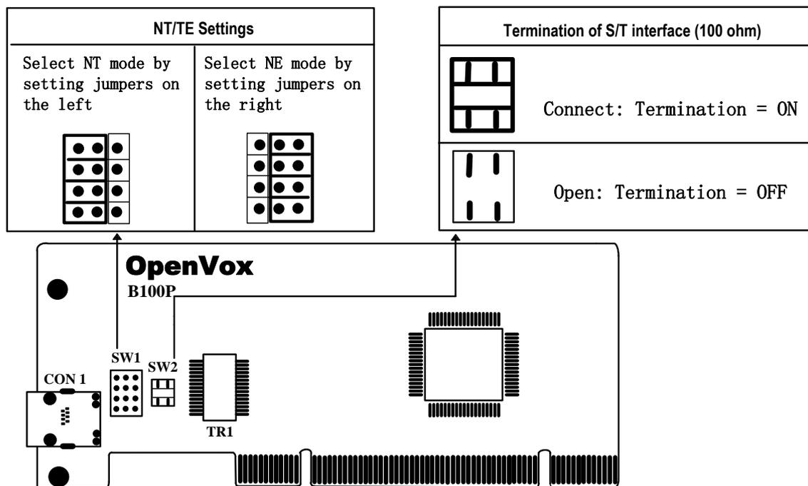
Figure 3 Jumper setting
